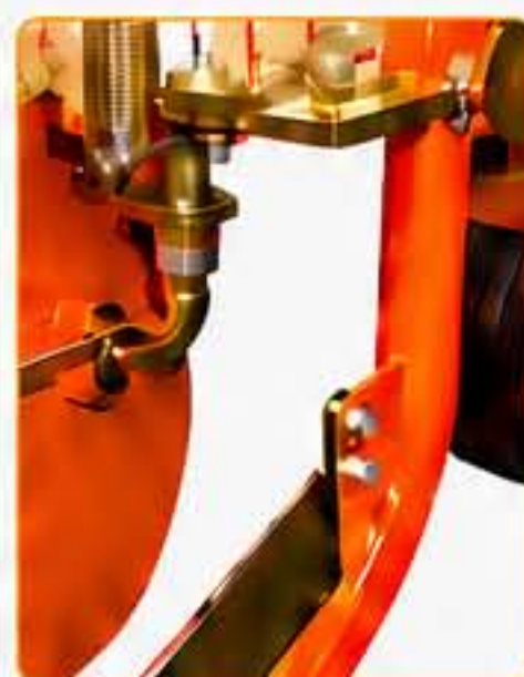
FURROW OPENER DISC Efficiently opens the furrow for the tape.
