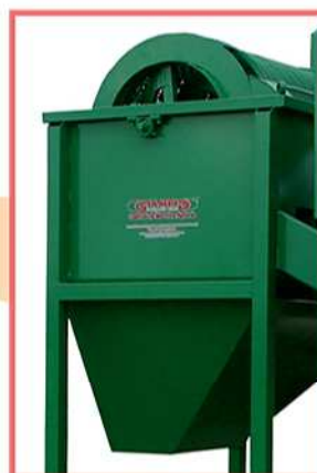
Passage in the rotating sieve with the ejection of a large part of the disposable material
