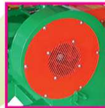
Fan increase with internal centrifugal clutch
