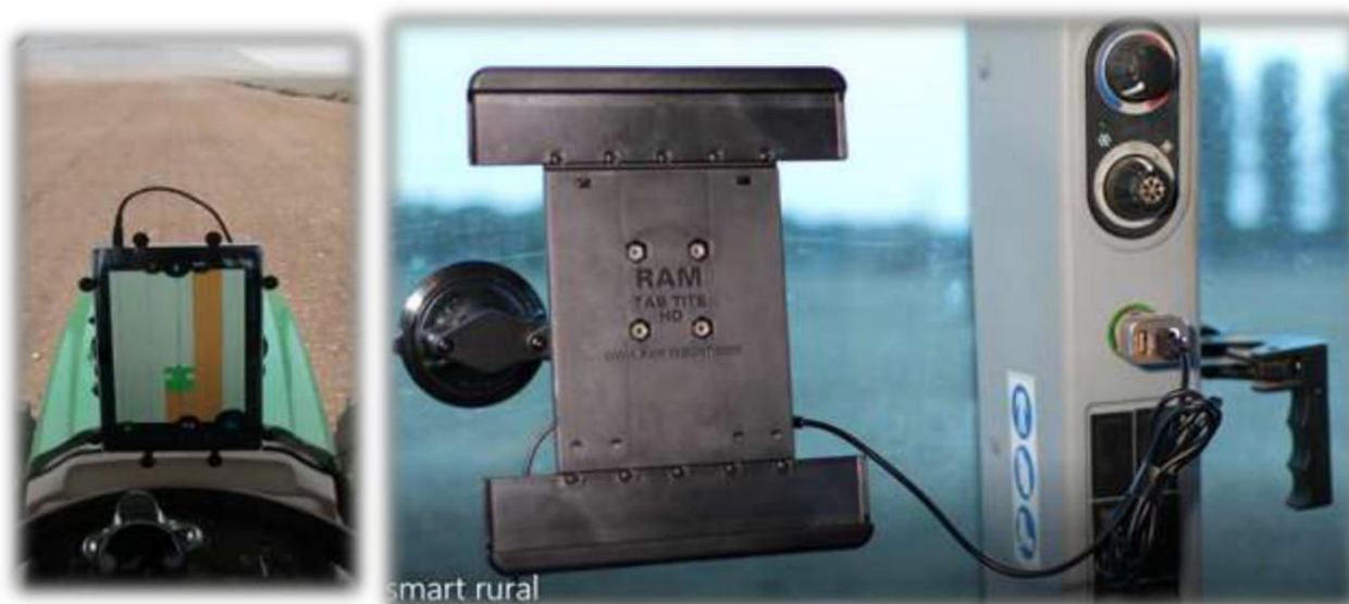
(Fig. 3-Connecting the Tablet to the tractor's cigarette lighter with USB cable)
