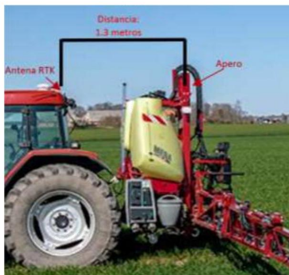
(Fig.18 - Adjusting the distance from the RTK antenna to the implement)
