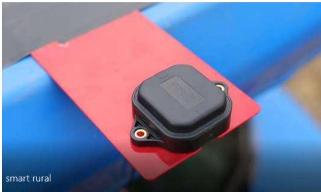
(Fig. 2-RTK antenna supported by metal plate)
