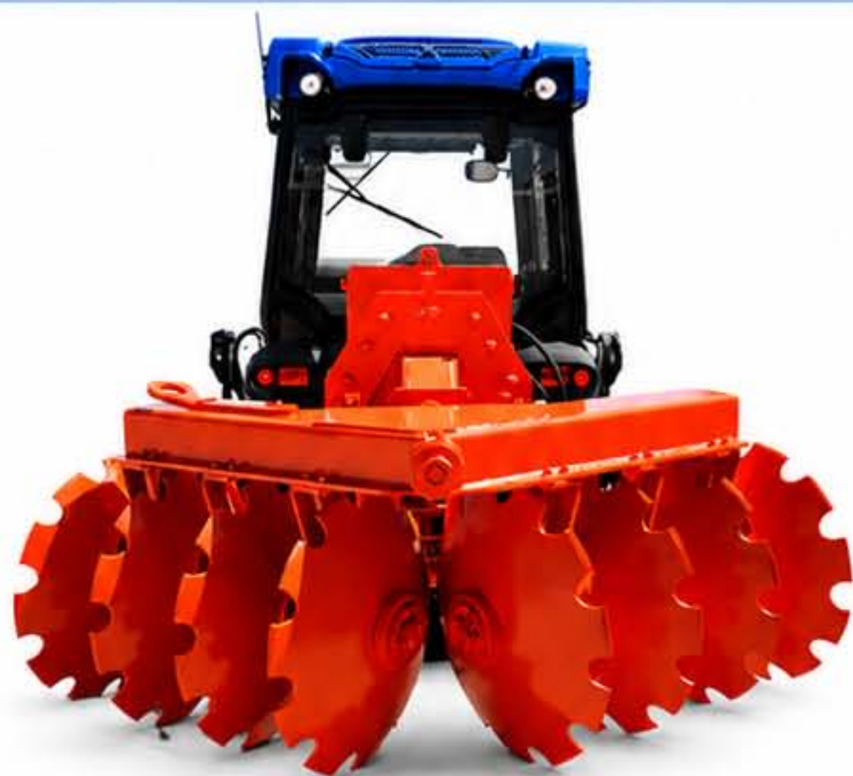
FI-GTVH/ER - V Disc Harrow with coupling to the rear implement carrier with quick hitch
