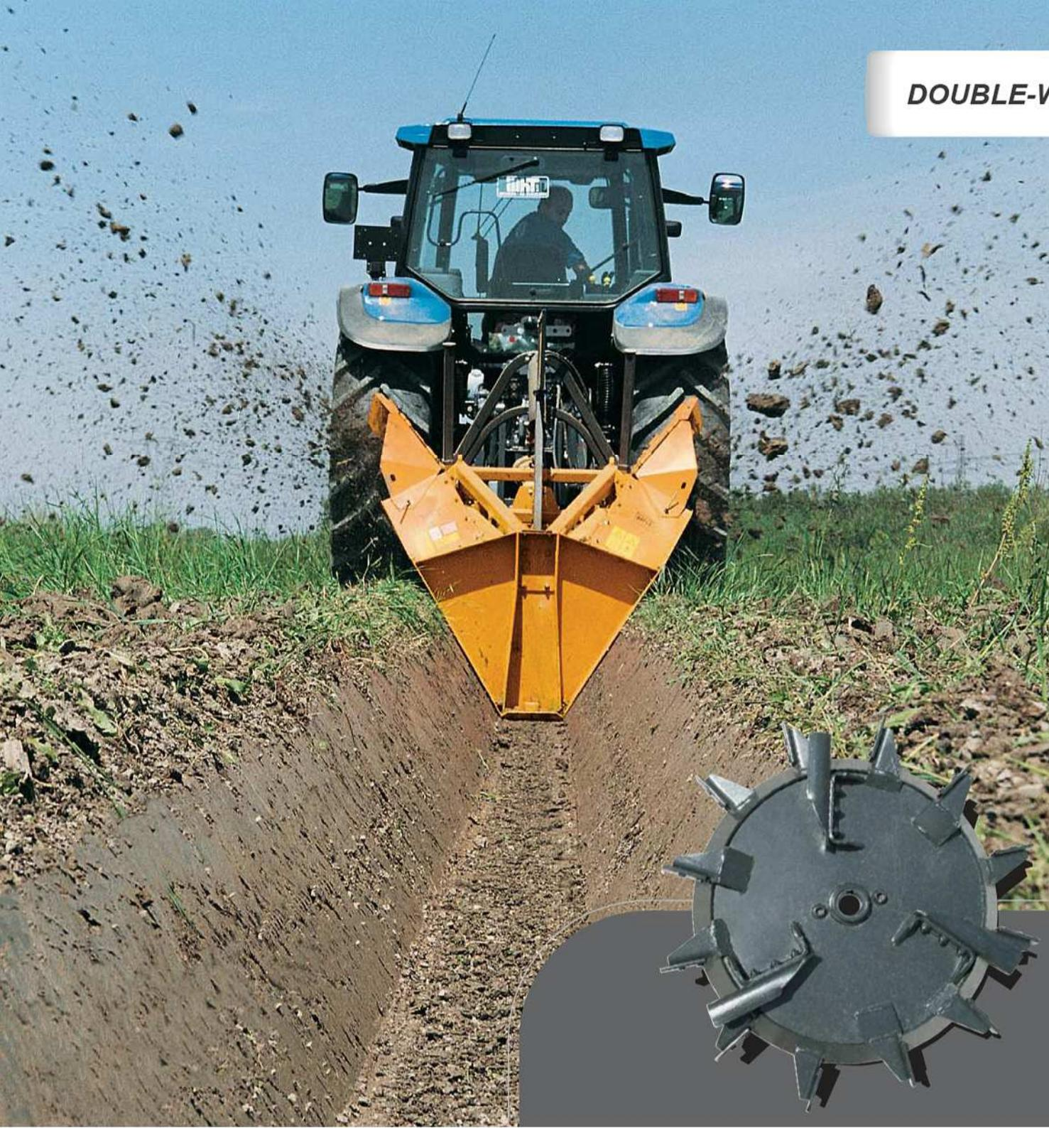
The double-wheell rotary ditchers are at the highest level in technology and performance for the creation and the maintenance of drainage and irrigation ditches.
