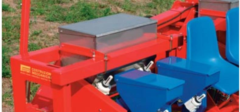
SPANDICONCIME E MICROGRANULATORE / FERTILIZER SPREADING BOX AND MICROGRANULATOR
