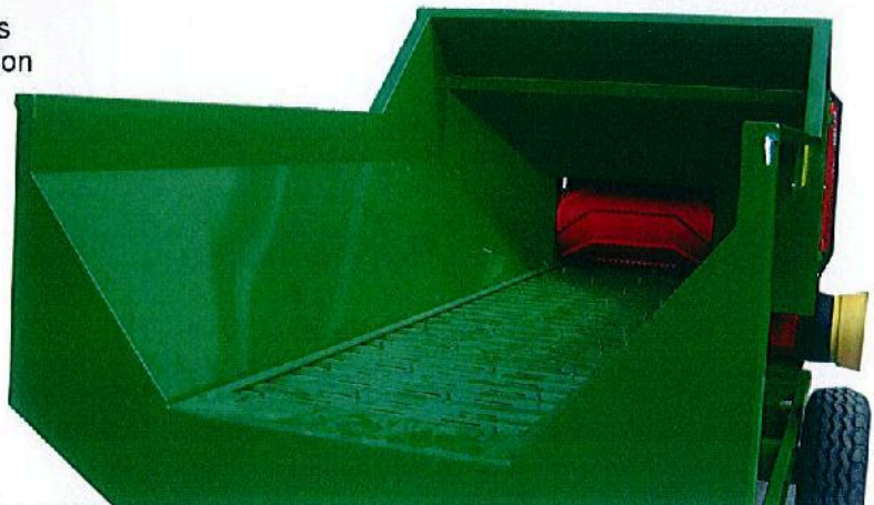
Hopper with steel loading belt sized 3000x1430x600 and hydraulic-powered feeding roller, both electronically controlled by no-stress device.
