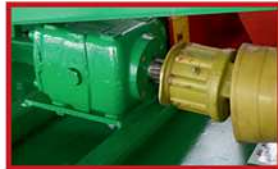
Box with power limiter in the presence of foreign bodies
