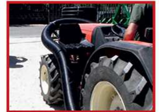
Fan boost with internal centrifugal clutch
